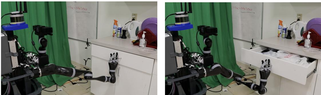
Figure 3.6: **Novel object manipulation.** A MOVO robot manipulating a novel drawer using a kinematic model estimated from a single depth image.
