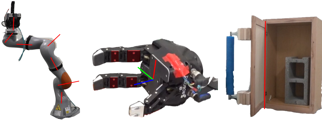
Figure 5.1: An example state that GARLA could encounter. The robot arm’s joints’ axes of rotation are displayed in the first image. The gripper’s frame is represented as a set of three colored axes in the second, along with tactile sensors highlighted in red. The articulated cabinet door’s axis of rotation is represented by a red axis in the third image.
