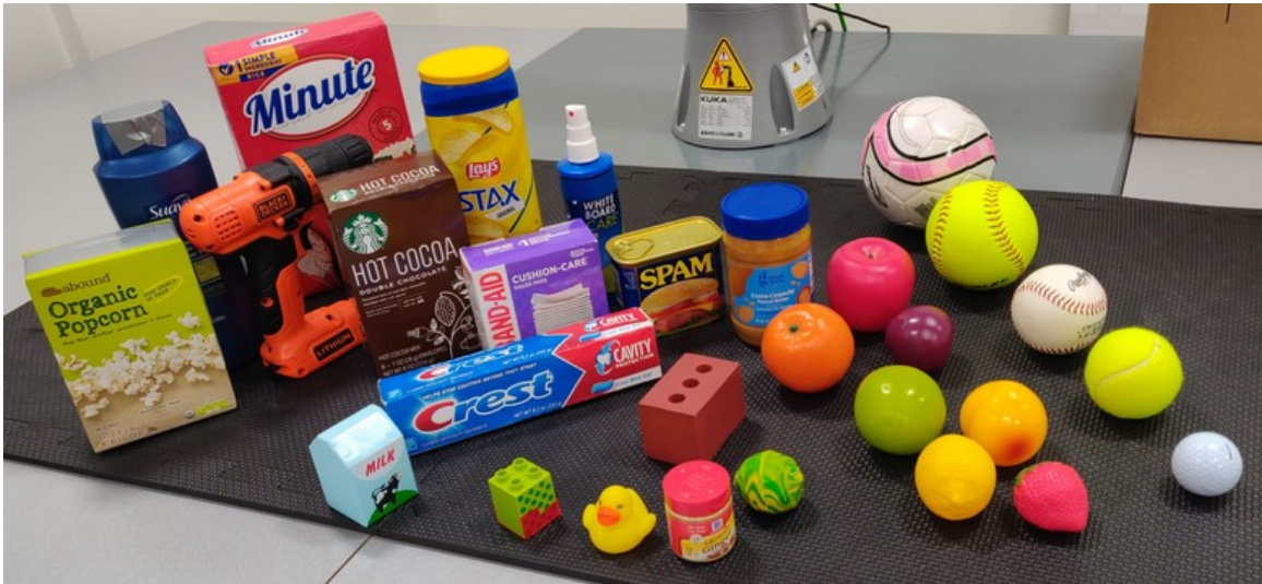
Figure 3.11: The set of objects MMGPD is tasked to grasp in the real-robot experiments. The six large objects on the left of the image are a shampoo bottle, a drill, a popcorn box, a cocoa box, a can of chips, and a box of rice. The 17 medium and six small objects on the right include fake fruit, sports balls, small toys, a box of toothpaste, a box of bandages, a jar of peanut butter, and a tin of Spam. Ten objects are selected from this set at random, and three random large objects are placed around a pile of the small objects to create a complex cluttered scene.
