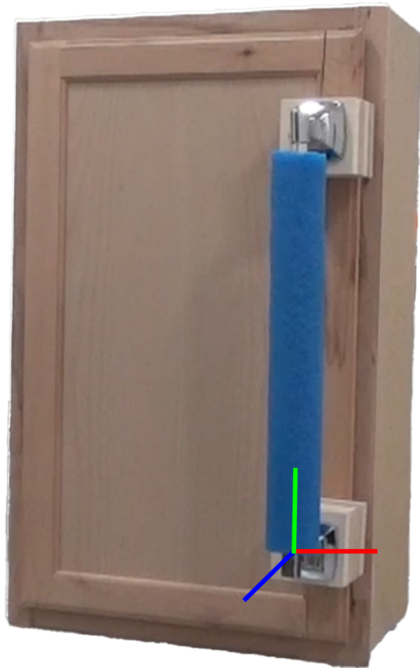
Figure 4.3: An example of the fixed frame of reference for the door handle. All poses passed to an ATOG classifier trained to open this door are represented in this frame.
