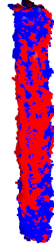
Figure 4.15: A point cloud showing all points on the graspable area of the door handle. Grasps centered at the blue points are in collision while grasps centered at red points are feasible.
