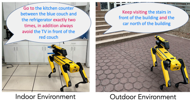
Fig. 1: Our system Lang2LTL-2 grounds spatiotemporal navigation commands in indoor and outdoor environments. The spatial and temporal components of the example commands are highlighted in blue and red, respectively.
